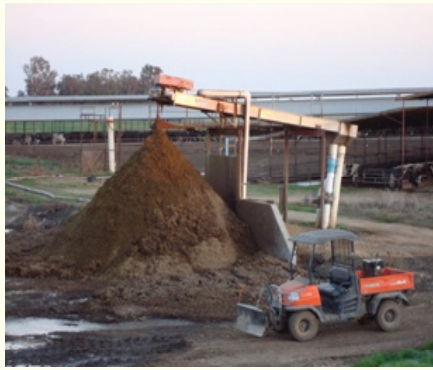
Figure 3. Manure Solids Separator.
